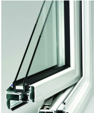
Double Glazing U Value-1.24 W/m 2 K
