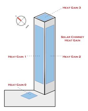
The total heat gain in the chimney is then calculated. Other inputs including the chimney inlet center height, chimney outlet/exhaust center height, the free area of both the inlet and exhaust of the chimney -with an equal value for both-, and the discharge coefficient value for the chimney are manually defined in this table.
