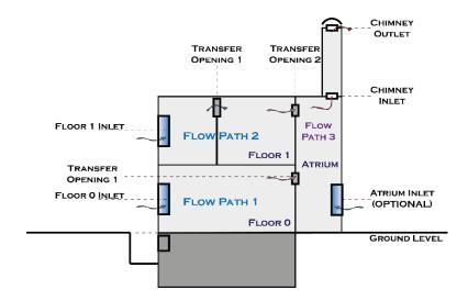
This is the case specific sheet where the flow paths are defined and modified in order to optimize the proposed openings in each path according to the pressure imbalance result shown as a YES/NO output under the column titled "Opening Size is Enough?".
