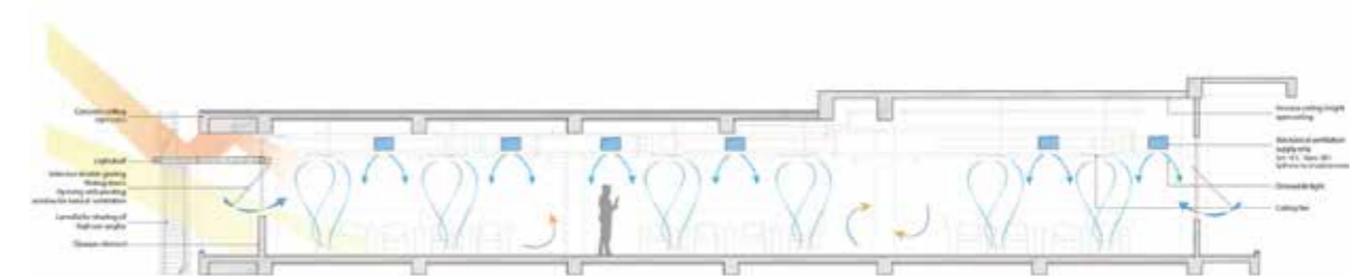
Fig 5.1.7 Typical section showcasing hybrid cooling concept elements such as the building facade working in conjunction with the MVAC system.
