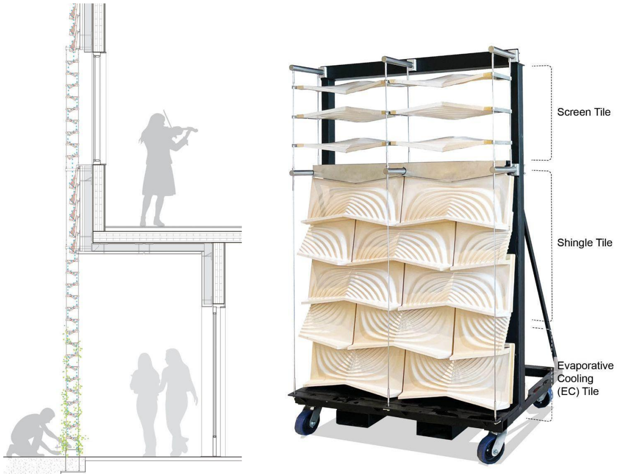
Figure 3. Left: Wall section with cross-laminated timber (CLT) structure, insulation, rainscreen cladding, and climbing plants. Right: Full-scale facade mockup.
